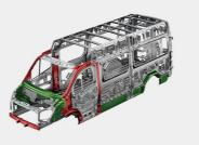
▶ The body framework made of high strength steel plates promotes the body stiffness by 20% than traditional body to better resist the impact load.
